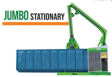
The **Ropax** "Jumbo Stationary Compactor is an innovative single container compactor that increases compaction in open top roll-off containers, allowing up to five times more discarded material in a single container. Due to the continuous rolling movement of its 4,000-pound spiked compaction drum, the material discarded is broken, torn and compacted up to five times the original volume. It is ideal for wood pallets, crates, cable reels, and bulky / voluminous waste.
